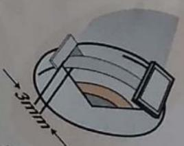
*Do be sure work rest is properly adjusted 1/8" (maximum distance) far from the wheel face.*
